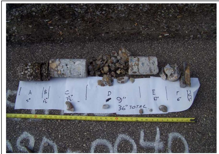
Test Length 4" Correction Factor .87 Diameter 3.95" Area 12.25 sq. in.
