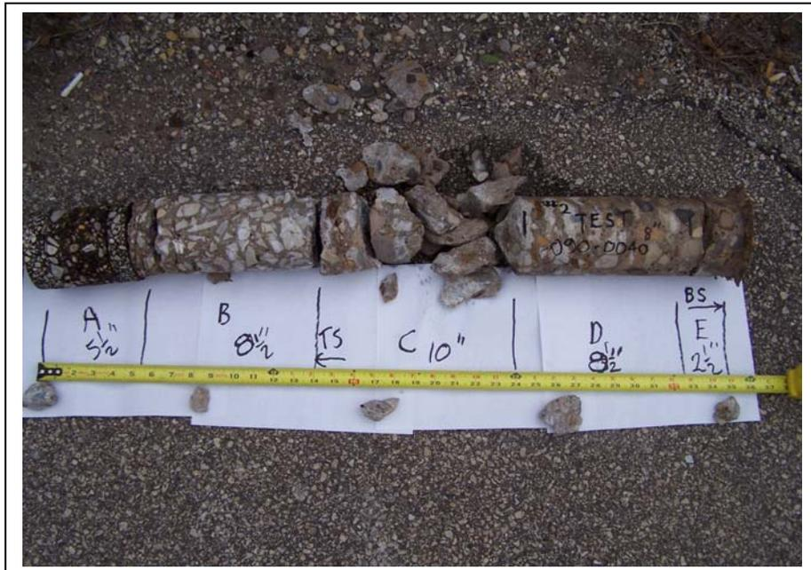
Test Length 7.75" Correction Factor 1.0 Diameter 3.95" Area 12.25 sq. in.
