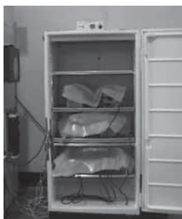
Monitoring and testing of UPS units at subfreezing temperatures in a freezer.
