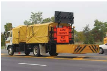
This photograph shows a truck-mounted attenuator attached to the rear of a large truck used in mobile work operations. This photograph was taken in daytime to show details of the truck and attenuator, but it is suitable for night operations.
