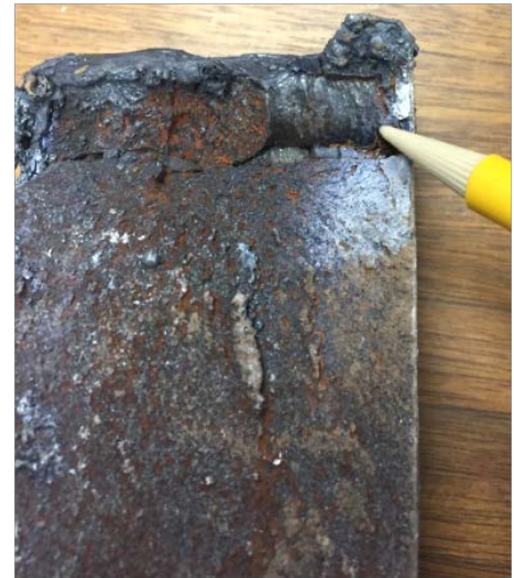
Figure 7 Sample taken from North Flange fracture surface. (HNTB)
