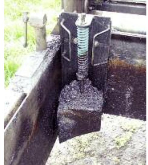
*This edging device—known as a shoe—creates the 30-degree pavement Safety Edge<sup>SM</sup>. The shoe is easily retrofitted to existing paving equipment.*
