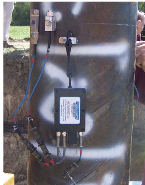
Pile Mounted PDA Sensors
