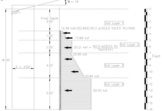
Figure 2, Soil Pressure Diagram
