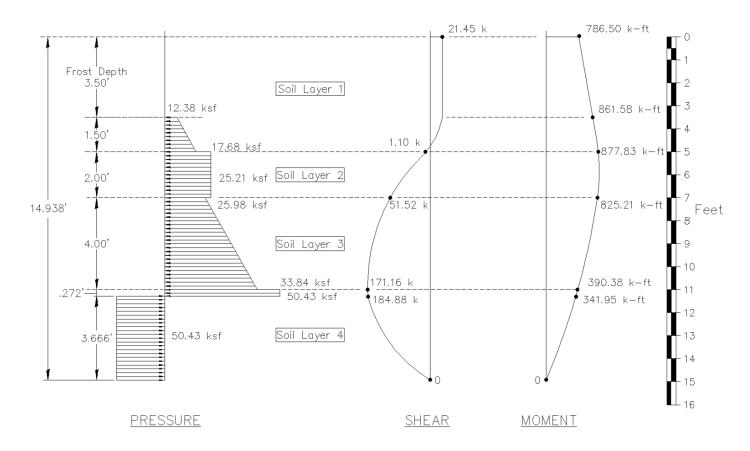
Figure 3.0, Final Design Soil Pressure and Shear Diagrams
