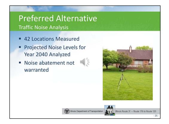
Existing traffic noise levels were measured at over 40 locations throughout the project area. Projected noise levels based on year 2040 traffic were analyzed using the FHWA Traffic Noise Model software which concluded that traffic noise abatement walls are not warranted.
