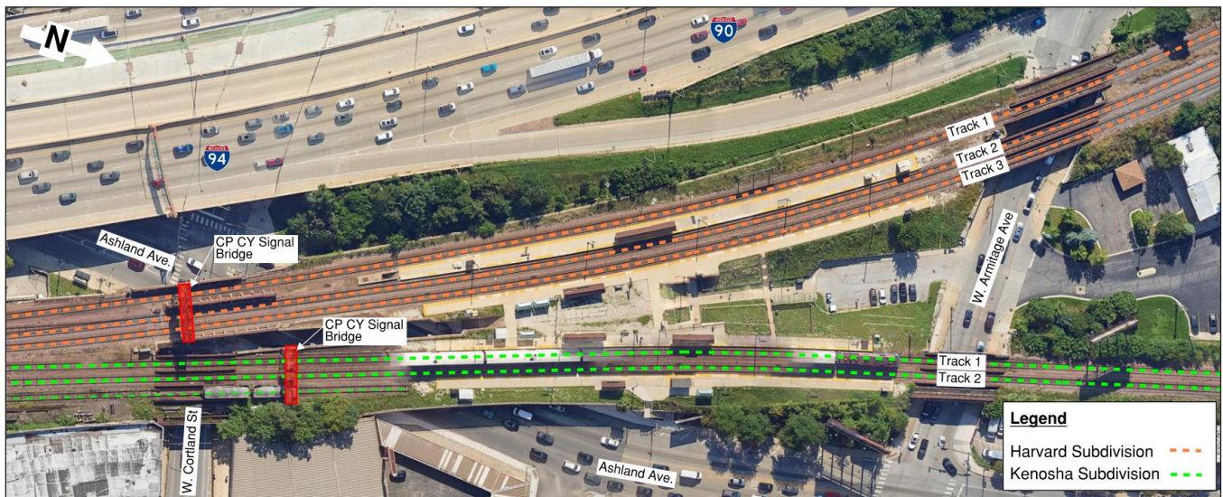
Figure 20: Clybourn Station Track Configuration
