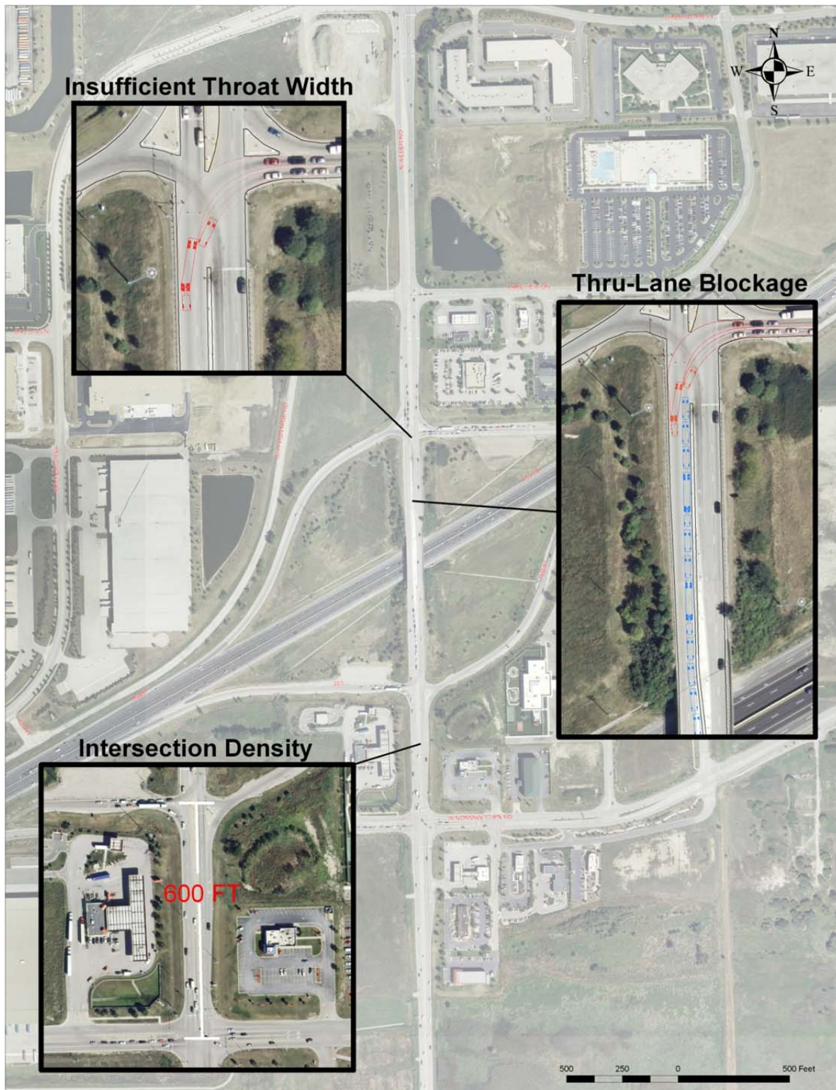
Figure 8. Project Area Operational Deficiencies
