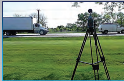
Traffic Noise Field Measurement
