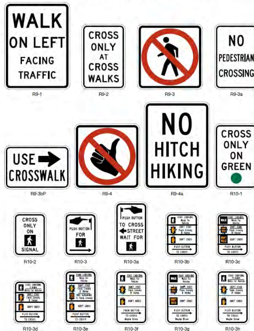
Figure 2B-27. Pedestrian Signs and Plaques (Sheet 1 of 2)
