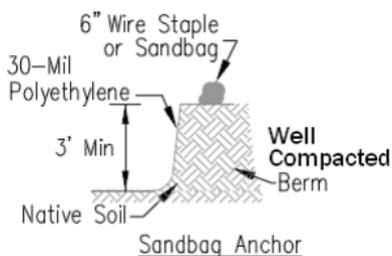
Earthen Berm Anchor Section
