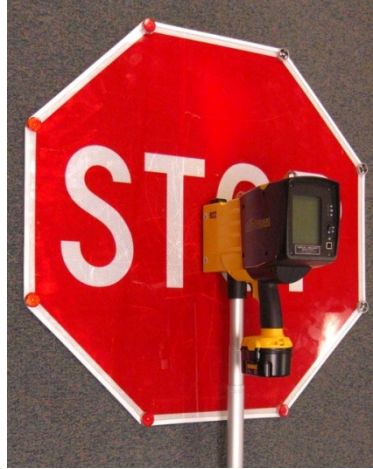
Figure 6-2 Taking a Measurement with the Pole Kit
