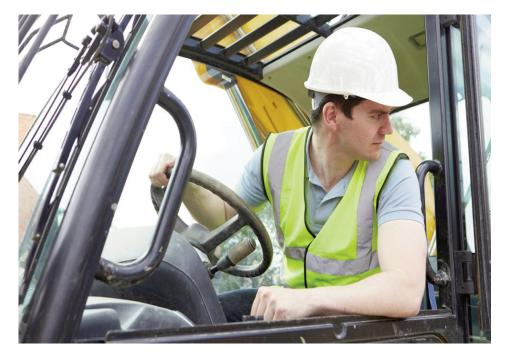
the vehicle and the area around it to assess possible blind spots, distances, height clearance, and the presence of any activity or workers that could interfere with a safe backing operation.
