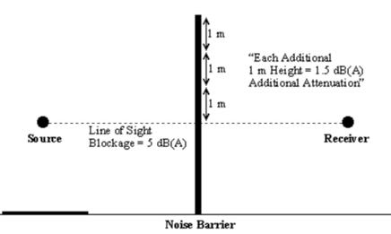
A noise barrier should not be designed at a height beyond that which is necessary to obtain the targeted level of noise reduction.
