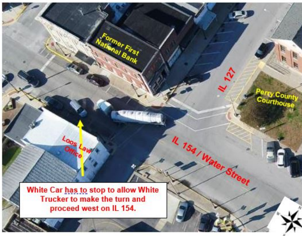
Figure 14 – Tanker Truck – Eastbound Lane Encroachment – IL 154
