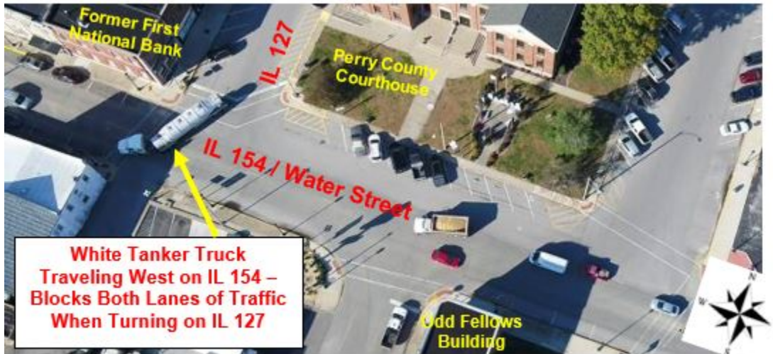
Figure 13 – Tanker Truck Blocking Both Traffic Lanes on IL 154
