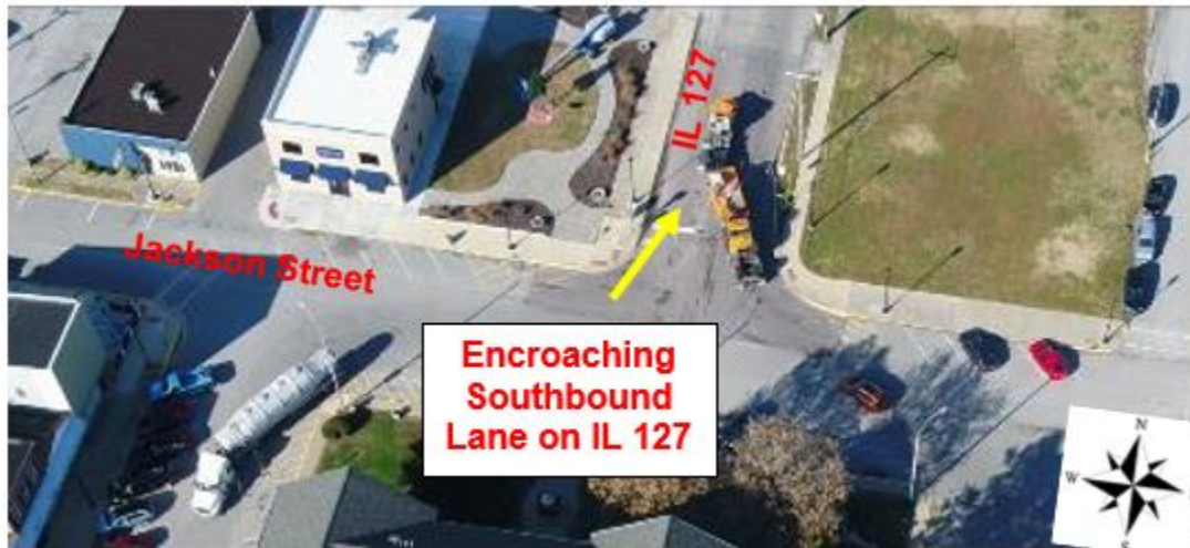
Figure 7 – Yellow Cab Truck – Southbound IL 127 Traffic Encroachment
