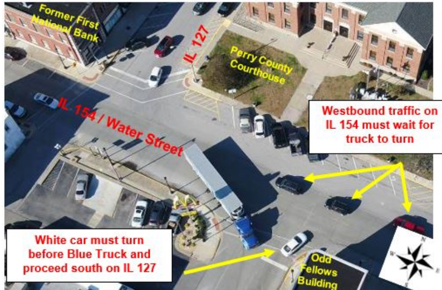
Figure 18 – Blue Truck Lane Encroachment IL 127
