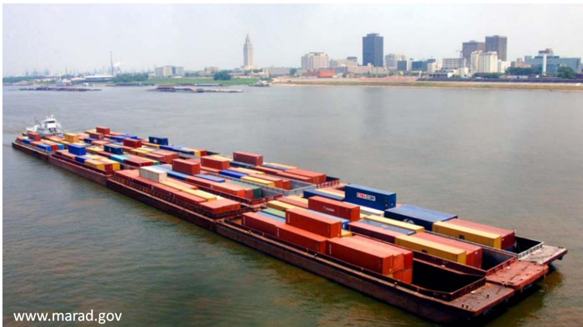
Figure 4: Containers Stacked in Standard Hopper Barges
