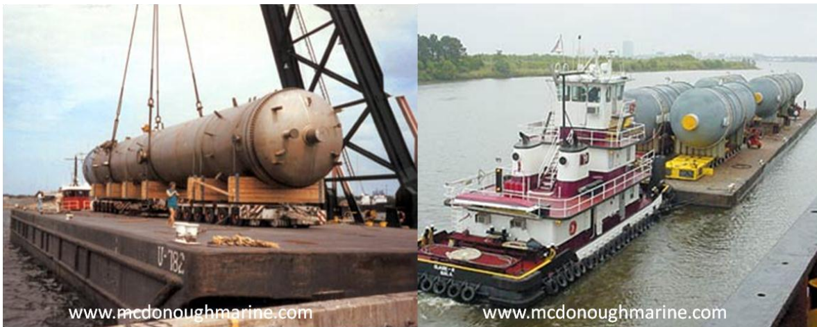
Figure 5: Heavy Equipment Cargo Rolled-on/Rolled-off Deck Barges
