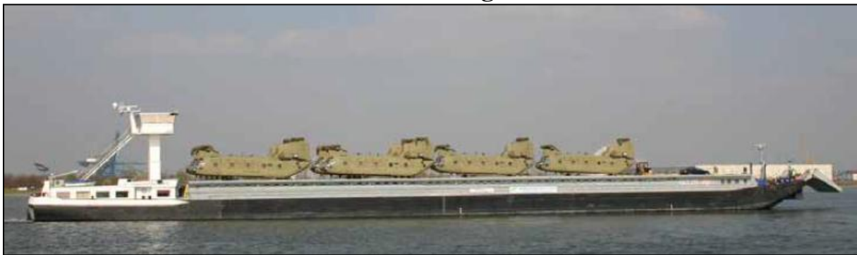
Figure 10: Examples of Self-Propelled Barges Operating in Europe Ro/Ro Barge
