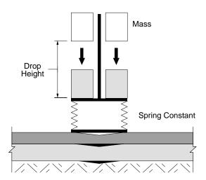
Figure 2: Load Applied to Pavement
