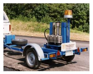
Figure 1: Falling Weight Deflectometer
