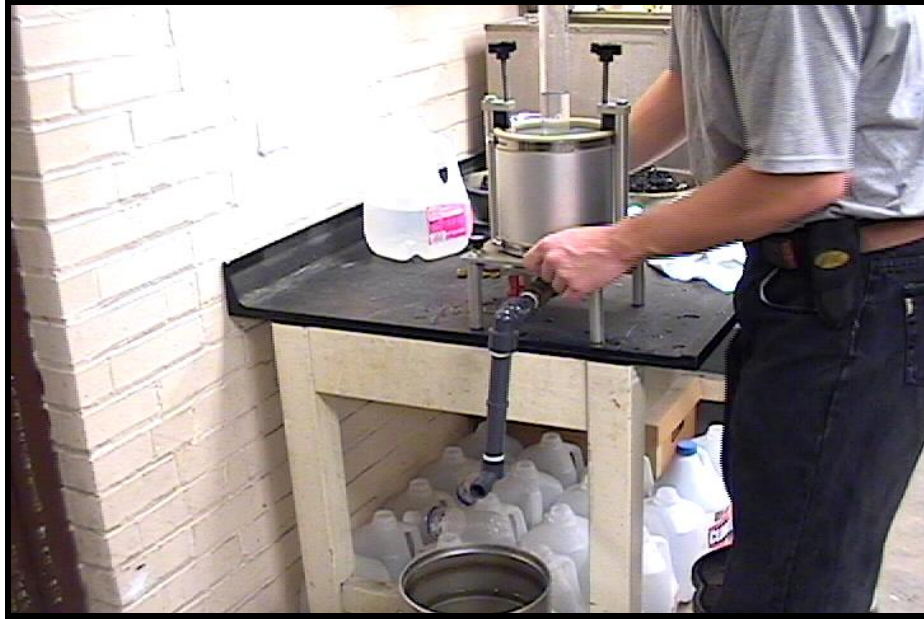
Figure 6: Preparing Lab Permeameter for Testing
