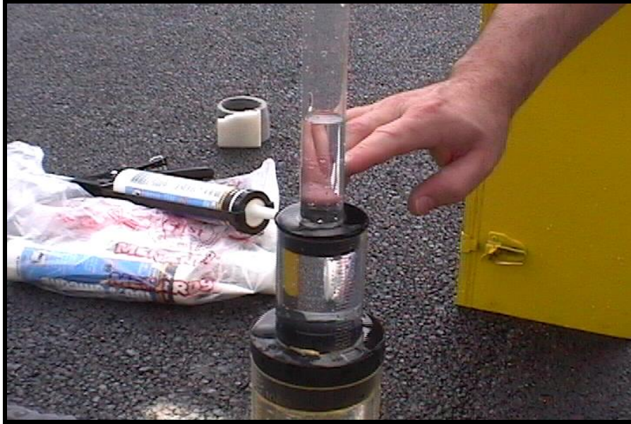
Figure 10: Measuring Water Fall in Standpipe
