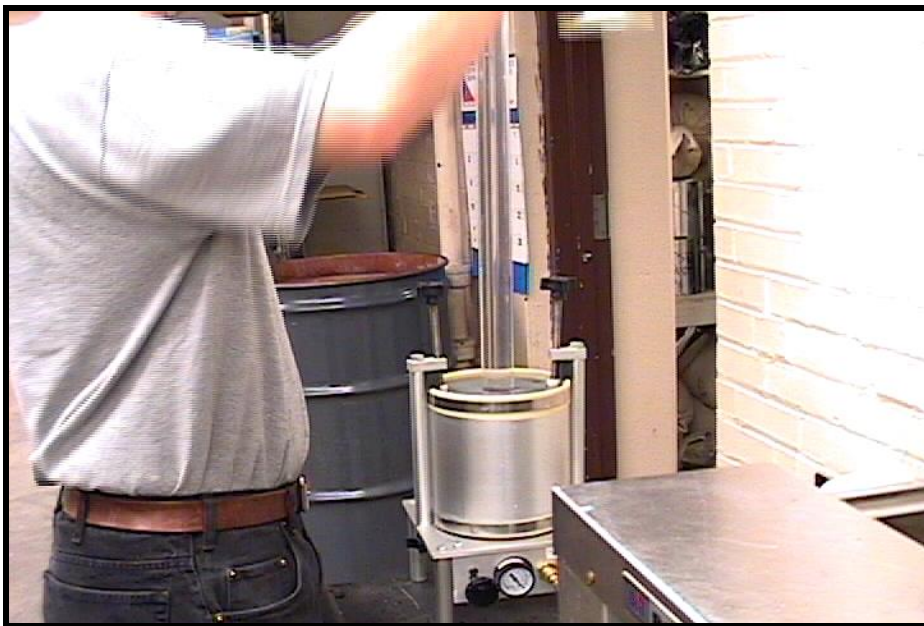
Figure 7: Timing Drop in Water Height of Lab Permeameter
