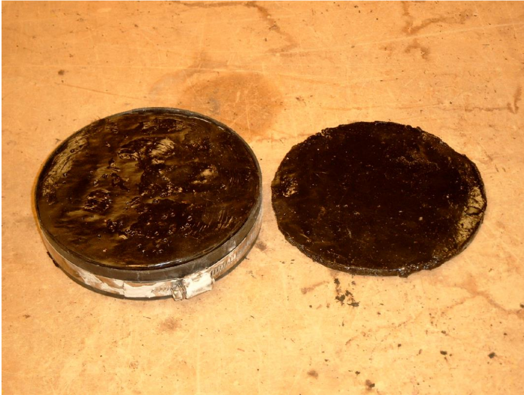
Figure 53: Joint Sealant Mold and Sample
