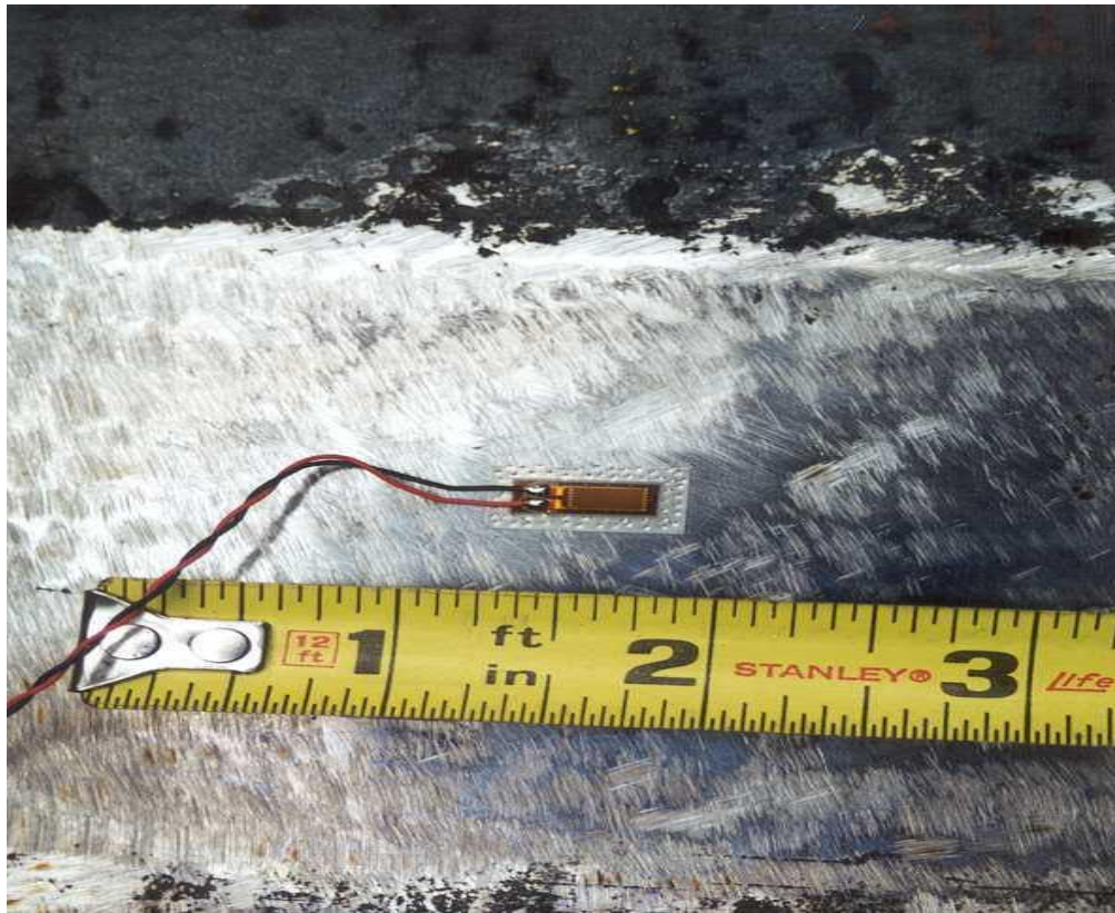
Figure 2. Pile gages were weldable quarter-bridge Micro Measurements strain gages supplied by Vishay Instruments. Gages are \frac{7}{16} in long and attached by micro-spot welding a \frac{5}{8} in long thin steel backing to a ground and cleaned steel surface. These micro-spot-welded gages are more reliable in translating strain from the steel substrate than with gages using bonding adhesives, which frequently debond during loading, or have limited fatigue life after sustaining frequent large strains during service.
