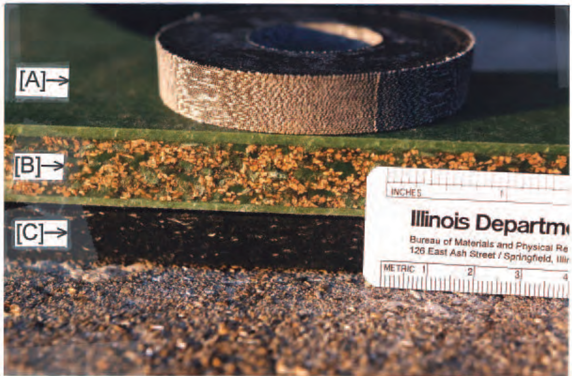
Figure 7. Close-ups of the cross sections of the Fabreeka®, Airloc 30 and SA-47 vibration attenuating material.
