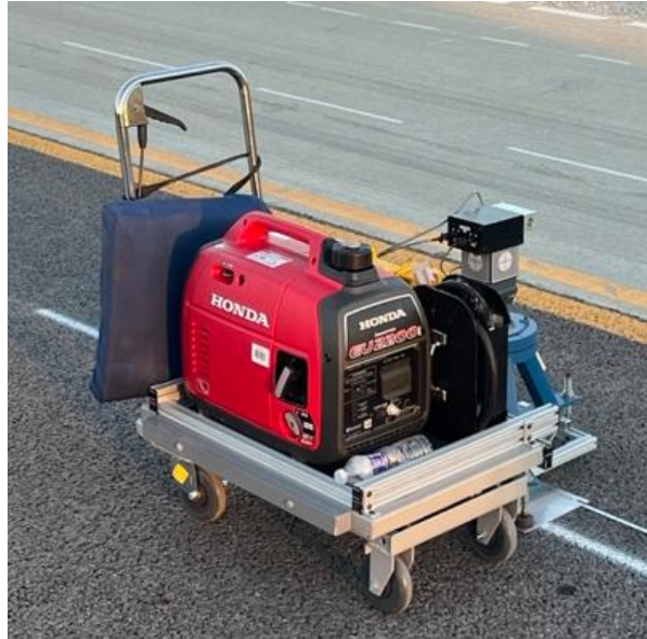
Figure 5. Gasoline generator for charging the BP.
