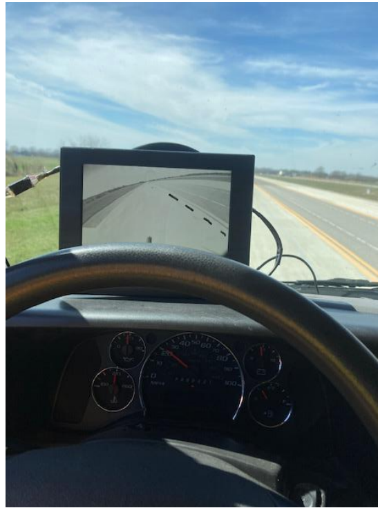
Figure 12. Dashboard monitor for lane tracking feedback.
