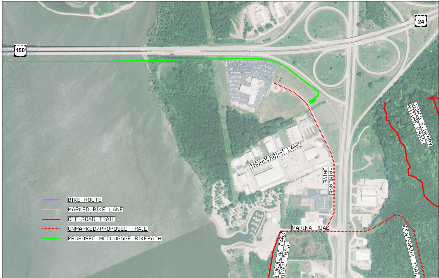
Figure 3.18 Eastern Interchange Multi-Use Path Connection
