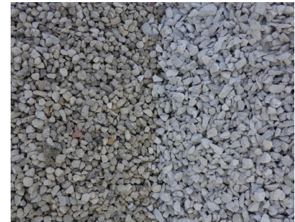
Slag (left) and virgin limestone aggregate side by side.
